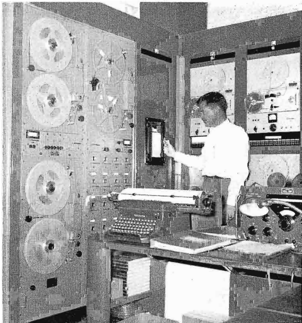
FIG. 44. R. H. Harrison, Assistant Chief Transmitter Facilities, at 24-hr. automatic-log of 15 transmitters. At left, note 14-channel continuous recorder.
